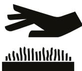
3. There is a relief image on the exhaust guard indicating that this surface can get hot. Particularly during and after operation/dri-ving the machine, there is a risk of burns.
