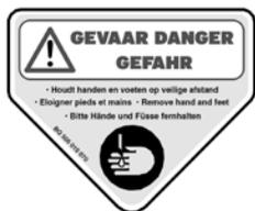
1. This sticker is affixed on the belt protection cover and warns about the danger of hand injuries. Keep your hands and feet away from underneath the machine as long as the blades are rotating. The engine must be turned off in case of faulty operation or before starting maintenance.
