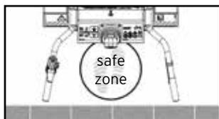
**Geometry of steering control:** When reversing the geometry of the handlebars reduces the risk of the operator becoming crushed between handlebars and an obstacle. In addition, the location of the joystick ensures that in this situation the operator's intuition and reflex will be to steer the machine in the other direction.
