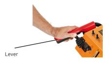
The lever is automatically set to the Slow drive setting. If the Fast setting is required, the selection lever should be moved to the left before depressing the dead man's handle.
