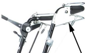
**Propulsion handles:** these handles are also on the handlebar and serve as actuator of the relevant wheel. Releasing the relevant handle will shut off the traction.
