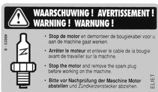
This sticker notifies the operator that the engine must be turned off and the spark plug cap removed before starting maintenance on the machine.
